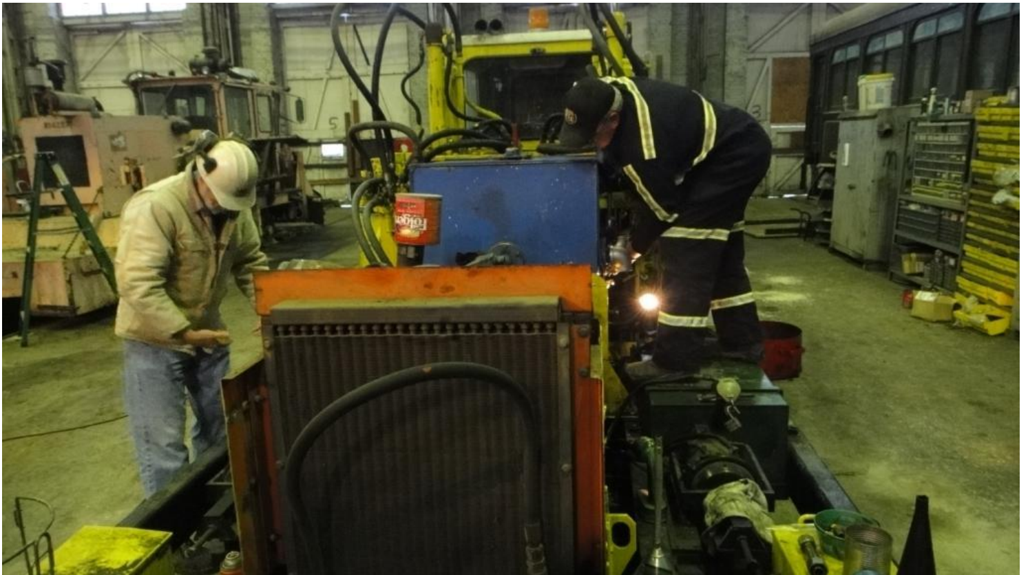
Alan and Scott work on rebuilding the tie-shear
